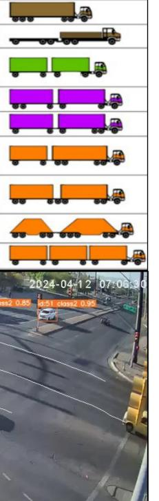
Used YOLOv7 to train an object detection model which has a mAP of 0.831. Combined detection and tracking result to implement counting algorithm based on typical trajectory annotation to assign each vehicle to different lanes. Below is the trajectory matching result for typical trajectory 0. Using camera calibration to achieve robust counting results based on 3D tracking.
